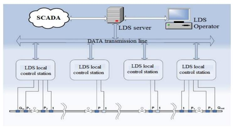
Volume balance method provides detection of of a leak equal to 0.75 - 1% from total flow. For instance, for a pipeline with D500 and flow 1100 m3/hour, the LDS will detect  $\sim 8$  m3/hour.
